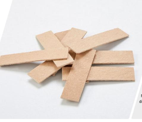
Glazing blocks are flat board cuts that are used in fire protection glazing to maintain the dimension and angle of the component. To do this, the blocks are wedged beneath the glass panes at two diagonally opposite corners in the window structure. Fire protection glazing blocks are heat-resistant and dimensionally stable.
