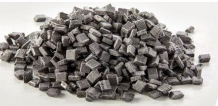
The profiles of the KERAFIX® Everseal series are flexible fire protection seals with a proportion based on expandable graphite. The expandable graphite proportion foams up in case of fire and increases its volume to seal fire doors or structural openings and prevent the spread of fire, for example. KERAFIX® Granulat NG-N series is used as the starting material for injection moulded parts that expand in case of fire.
